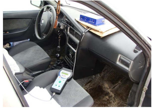
4 Picture: Sedan Nexia II ready for pavement roughness survey.
